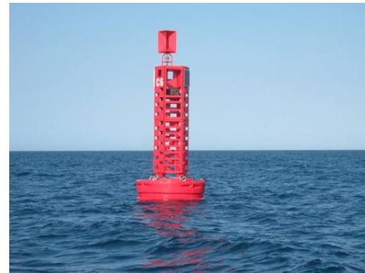
4. Replacing steel buoys with polyethylene
