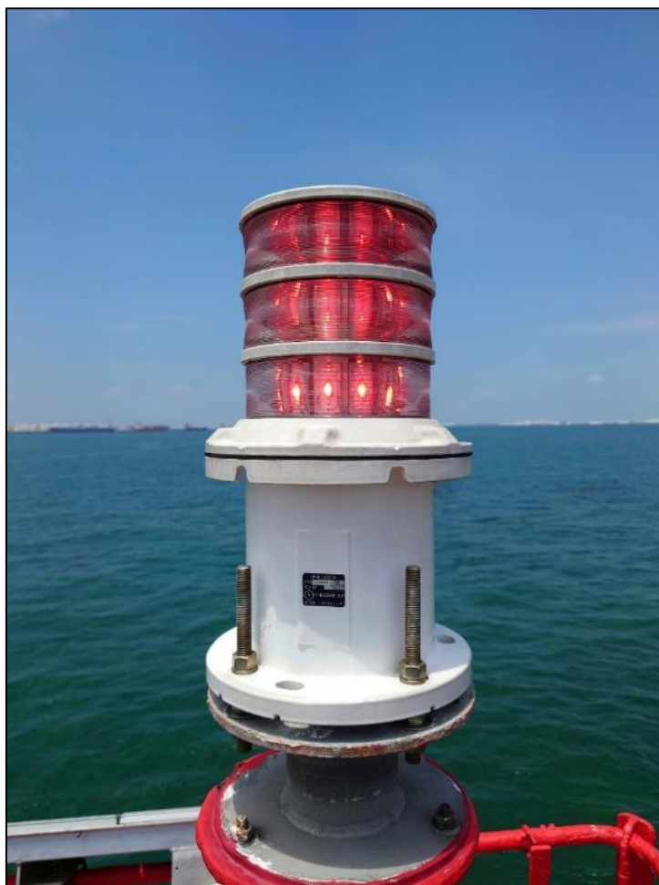
Figure 6: Prototype three-tiered Dual Intensity Lantern Installed During Phase 3 of Trial at Cyrene Beacon (High intensity flash)( FL.R.2,5s8m10M)
