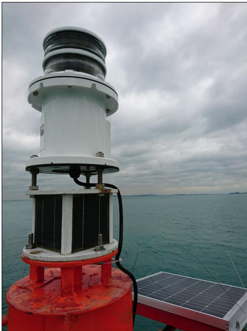
Figure 3: Prototype two-tiered Dual Intensity Lantern installed during Phase 2a of Trial on Sebarok Beacon (Fl.R.5s8m5M)
