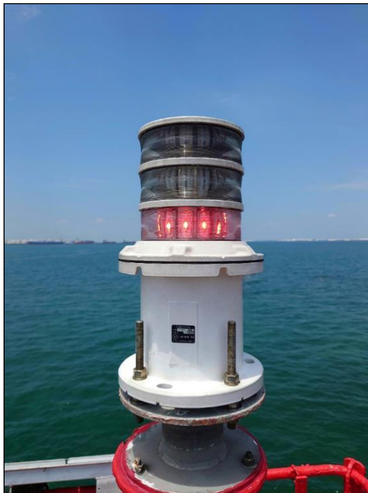
Figure 5: Prototype three-tiered Dual Intensity Lantern Installed During Phase 3 of Trial at Cyrene Beacon (Low intensity flash)(Fl.R.2,5s8m10M)
