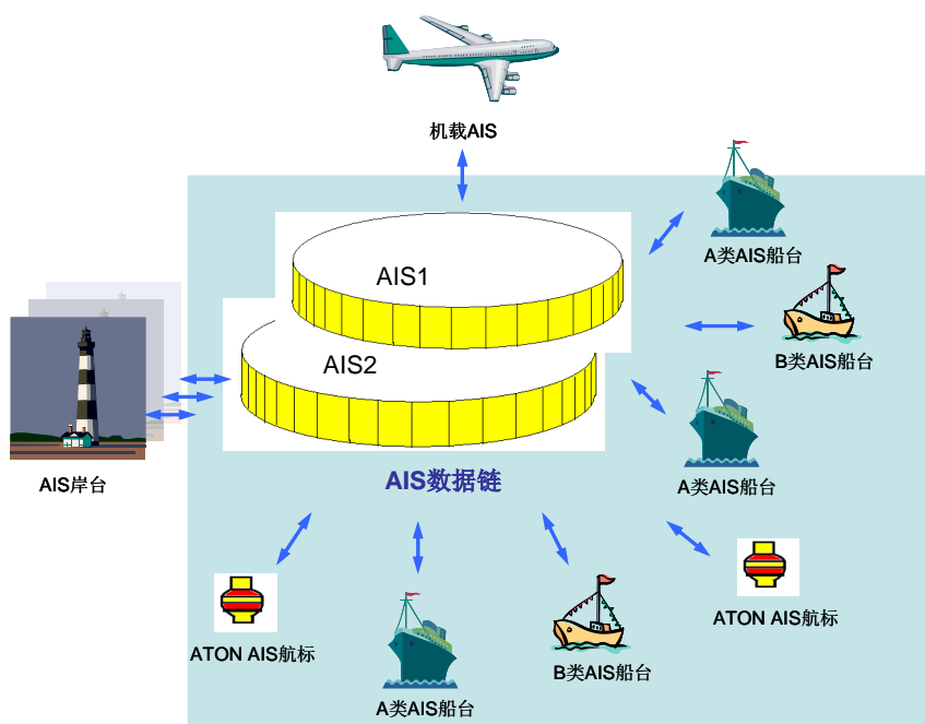
Figure 47: AIS system diagram
