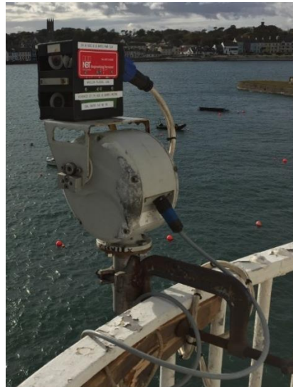
Figure 38 – One of GRAD’s field measurement calibration lights mounted on a remote-controlled pan/tilt head, with the whole assembly clamped to Donaghadee Lighthouse (Northern Ireland) balcony handrail.
