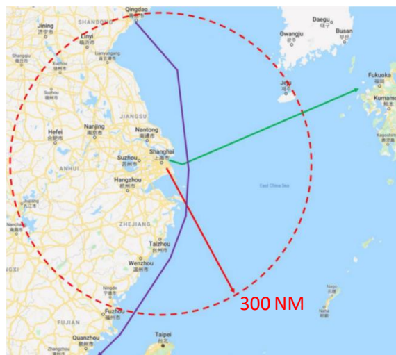
Figure 3: area covered during NAVDAT 500 kHz test in Shanghai, China
