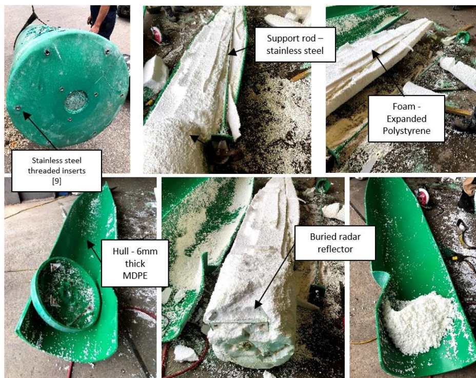
Figure 33: The dissection of current monocoque plastic buoys
