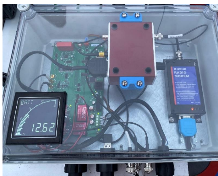
Figure 42 – The new field measurement data capture and communications unit.
