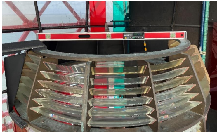
Figure 50 – Spirit level showing the axis of tilt of the Needles Lighthouse optic.
