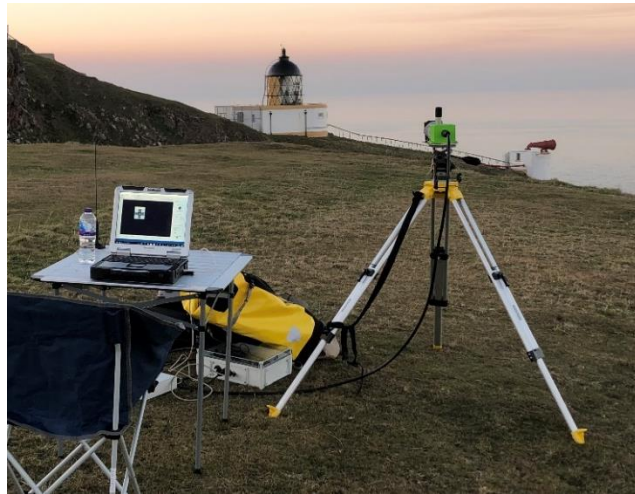
Figure 40 – The green enclosure of the new SiPM mounted on a tripod during a field light measurement at Saint Abbs Lighthouse, Scotland.
