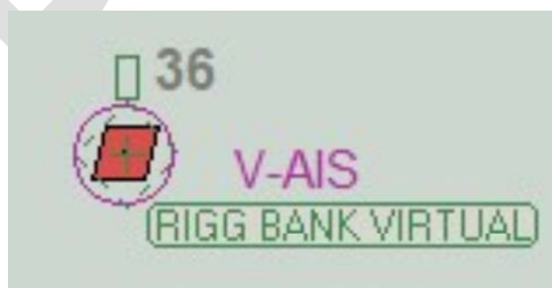
Figure 9 Broadcasted Virtual AIS AtoN port hand mark symbol displayed over the IHO ENC charted symbol
