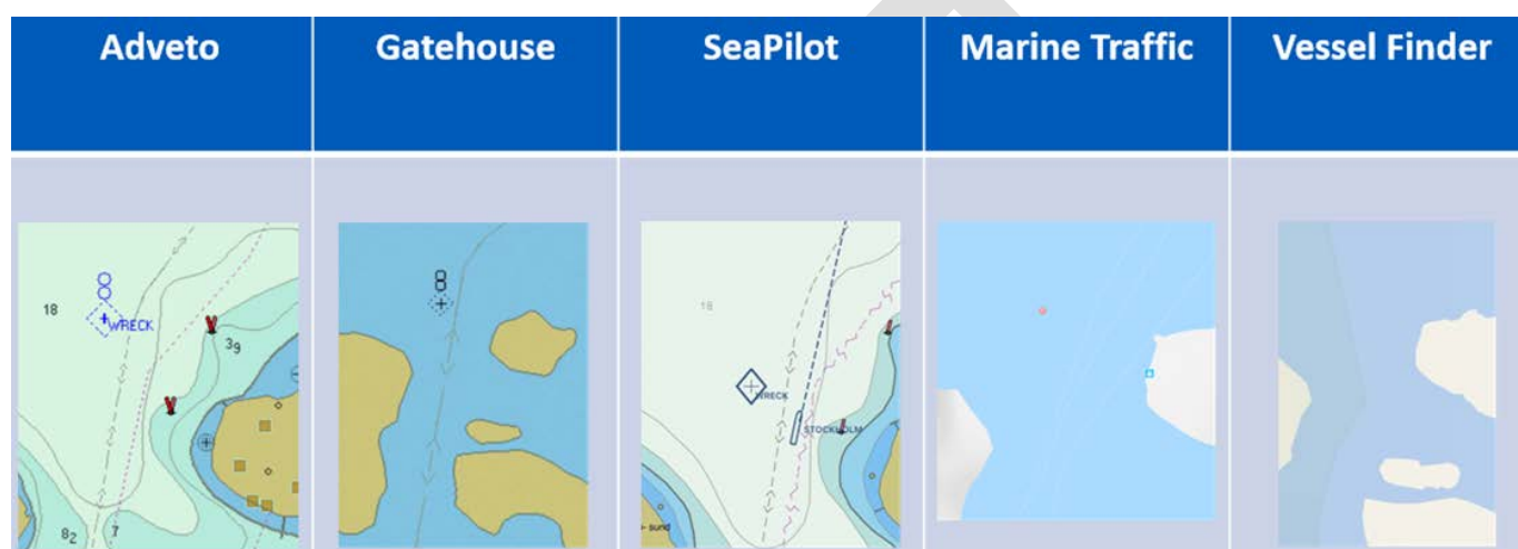
Figure 2 Variation of imagery due to software and type of ECDIS equipment or mobile application
