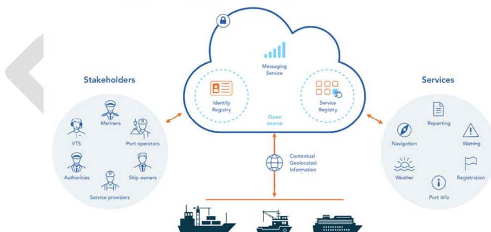
Figure 2 Figure 1 MCP Components for setting up a platform for the provision of maritime services in the context of e-Navigation
