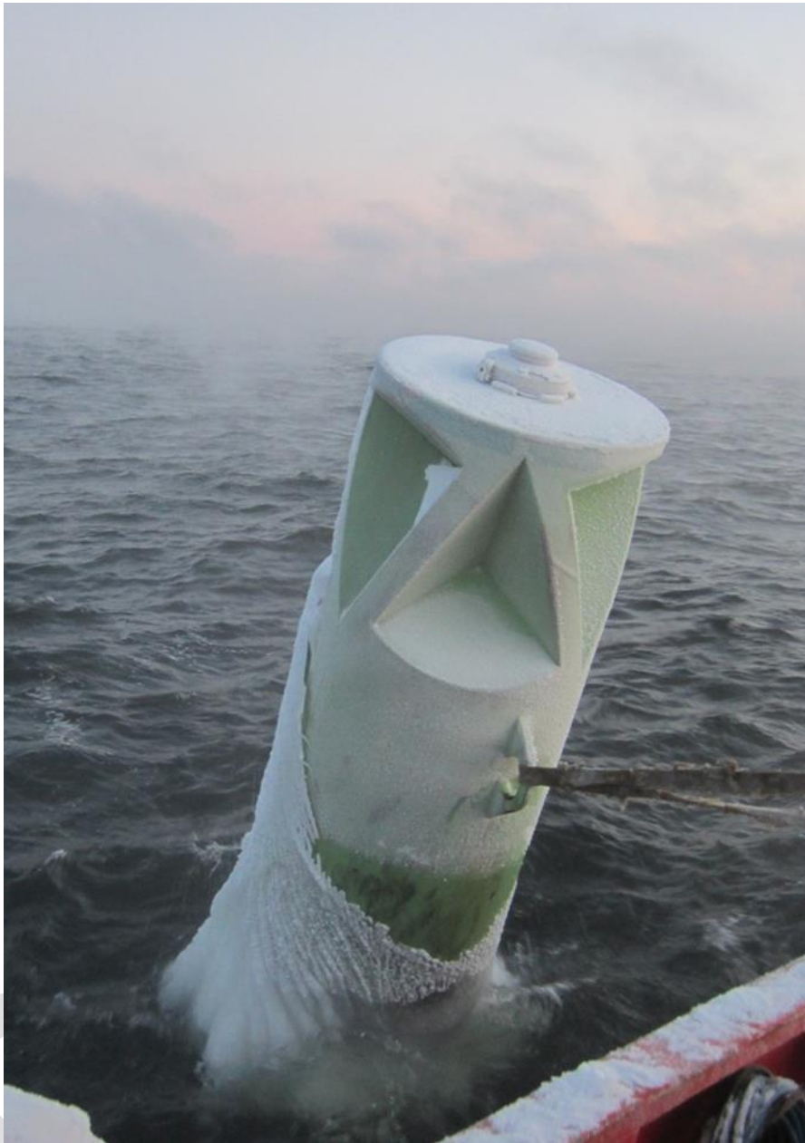
Figure 6 Buoy (and light) covered in ice
