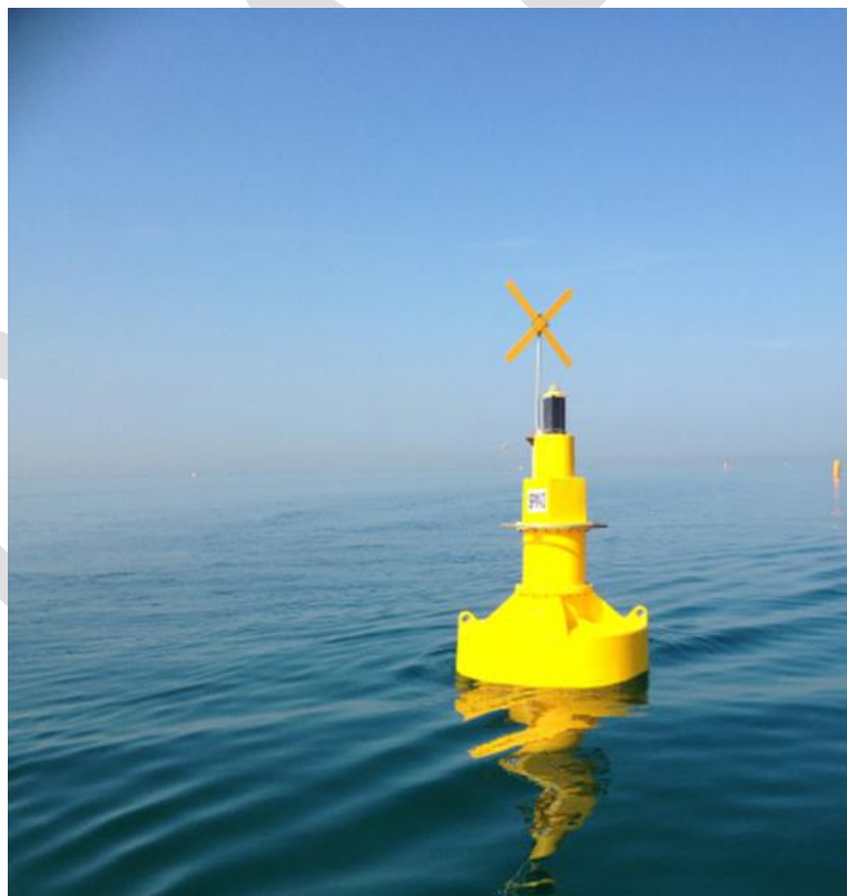
Figure 12 Overcoming background lighting with the use of colour and shape
