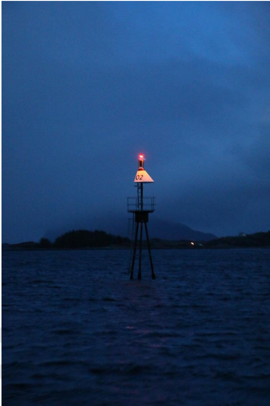
Figure 8 Night-time view – indirect lighting used on a beacon in Norwegian waters
