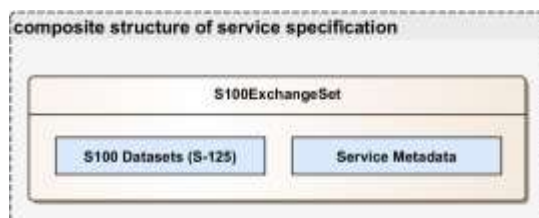
Figure 11: S-125 dataset coupled with service metadata in an S-100 Exchange Set.
