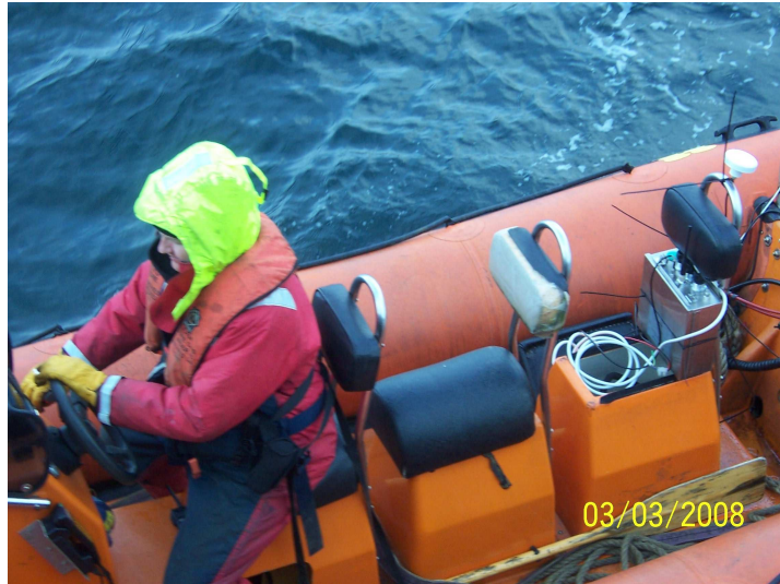
Figure 3: AtoN equipment mounted in the rear of an inflatable boat
