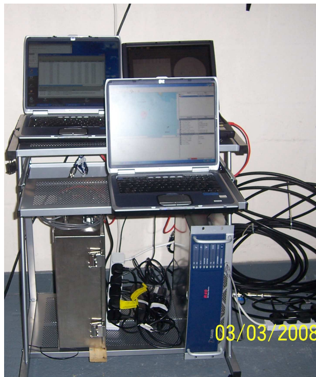
Figure 4: The shore side base station and equipment: AtoN monitoring, e-ANSI message generation and AIS base station
