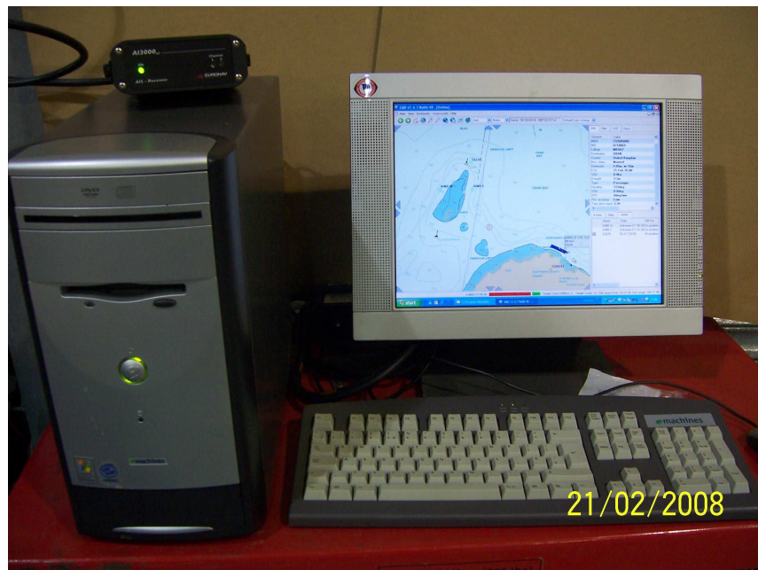
Figure 3: Ship station set-up: AIS unit and electronic chart display computer, showing the Oban Bay area; on the right hand side of the chart there is a text area listing various parameters of the selected AIS target.
