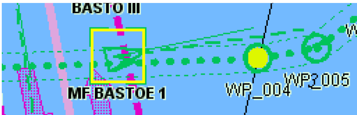
Figure 3. Suggested style of other ships intended route based on future way points transmitted by the other ship's navigation system.
