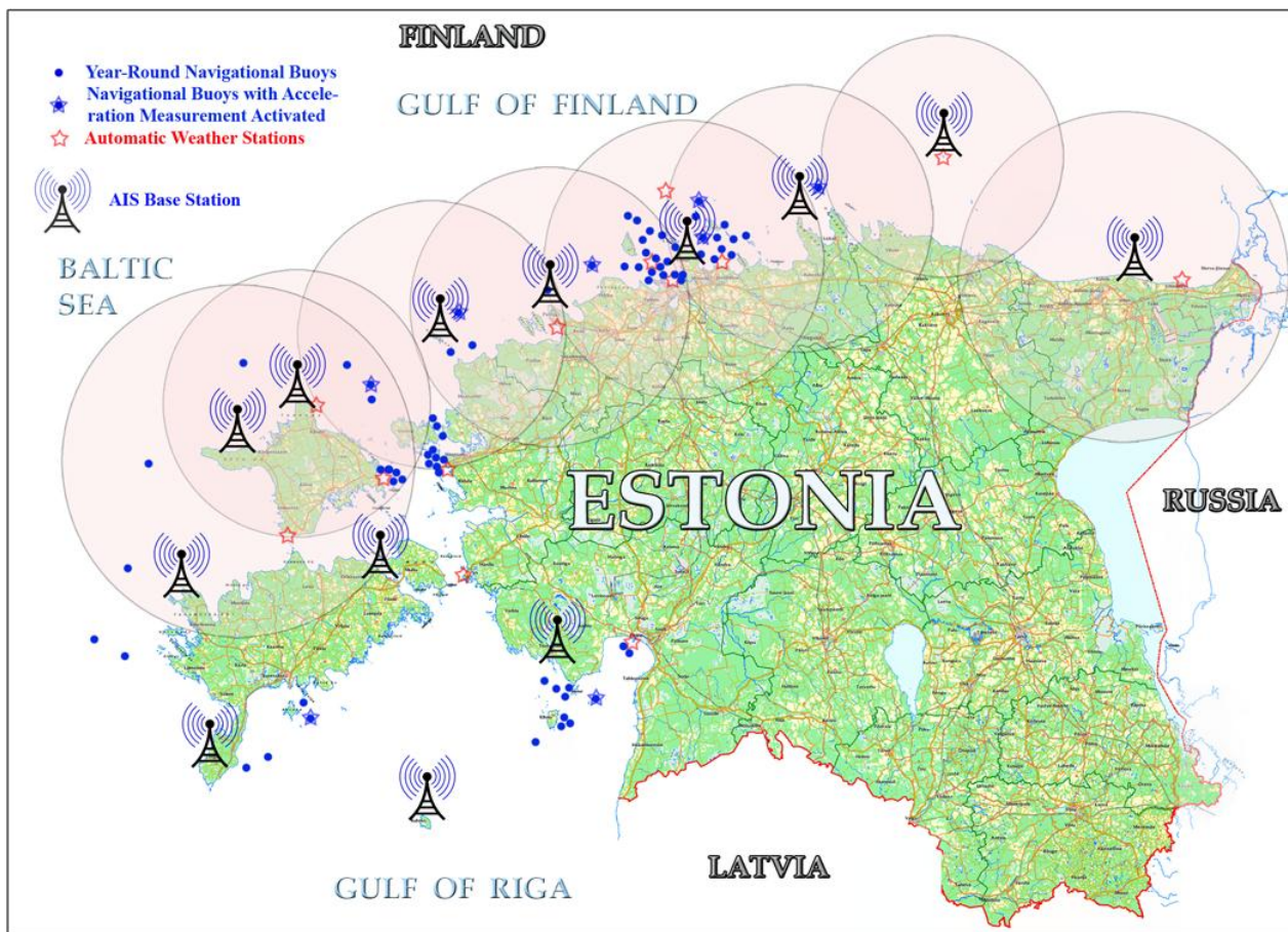
Figure . Established shore side AIS infrastructure of the Estonian Maritime Administration is mainly based on the “VHF for VTS” software/hardware solution developed and supplied by Cybernetica AS in 2004 for the mandatory Gulf of Finland Ship Reporting System area (GOFREP) in accordance with the IMO MSC approved traffic separation scheme (AIS base stations with radio coverage shown). GOFREP with its automated AIS report exchange between Estonian, Finnish and Russian authorities can be considered the first internationally interoperable e-Navigation project in the region. The AIS base stations without radio coverage shown will be integrated with the synthetic AIS signalling shore side infrastructure in 2011. Buoy stations marked by blue stars are candidates for becoming wave height measurement stations.
