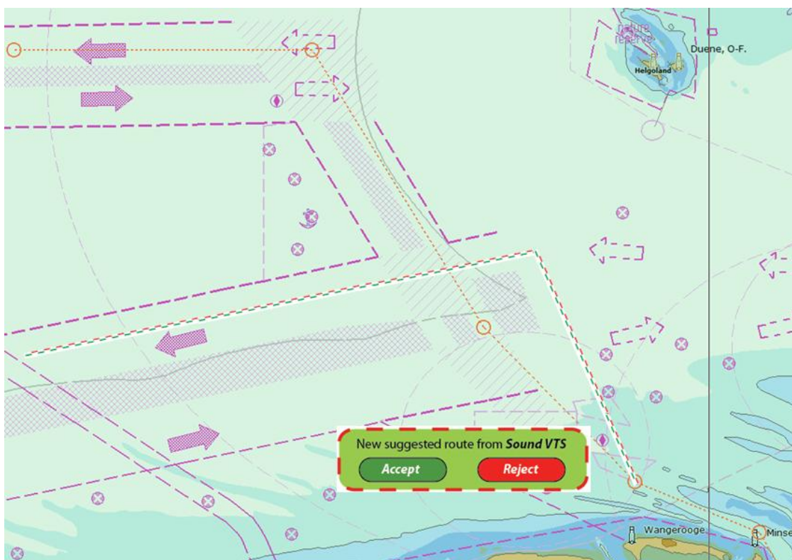
Figure 8. A possible scenario where the Elbe VTS has sent a new suggested route segment to a westbound ship. (NOTE: The Accept/Reject box could appear in the bottom menu of the display to avoid covering important information in the chart area).
