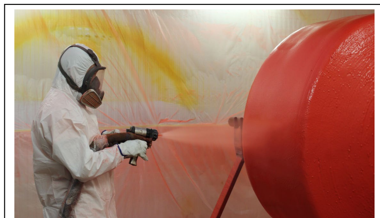
Figure 56: Coating of elastomer polyurethane
