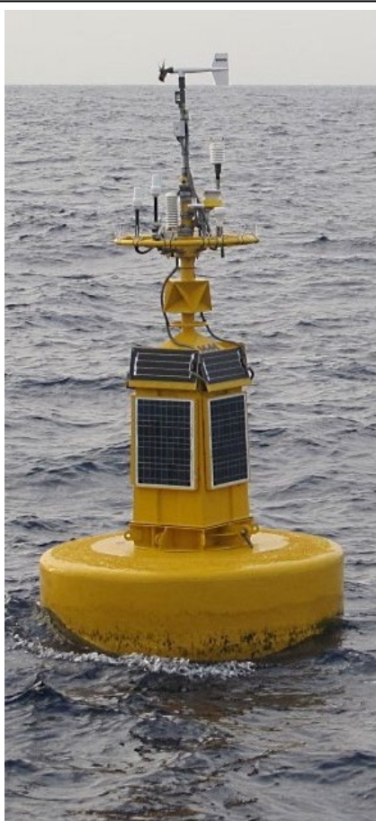
Figure 62: Solar and wind powered lit elastomer buoy with measurement equipment
