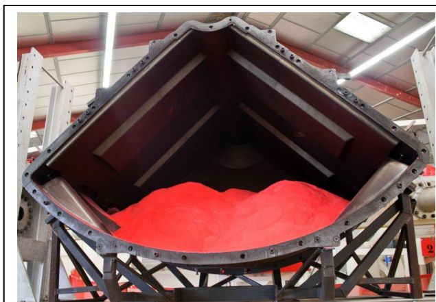
Figure 11: Mould filled with plastic powder
