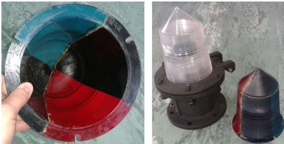
The green and red sectors need to be aligned with the buoy rudder.
