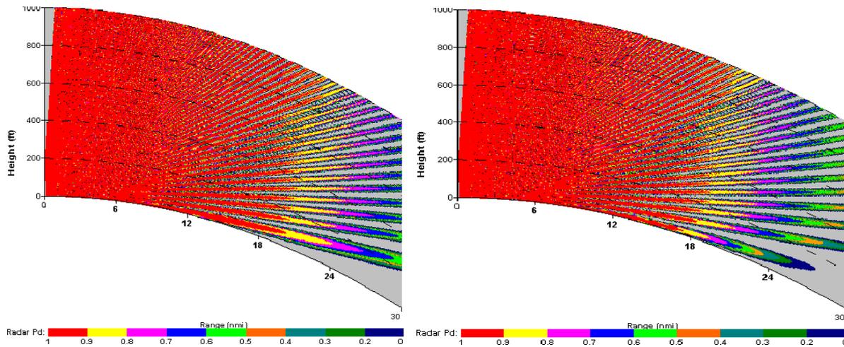
Figure 13 Coverage diagram, in standard atmosphere (left) and including an evaporation duct (right).
