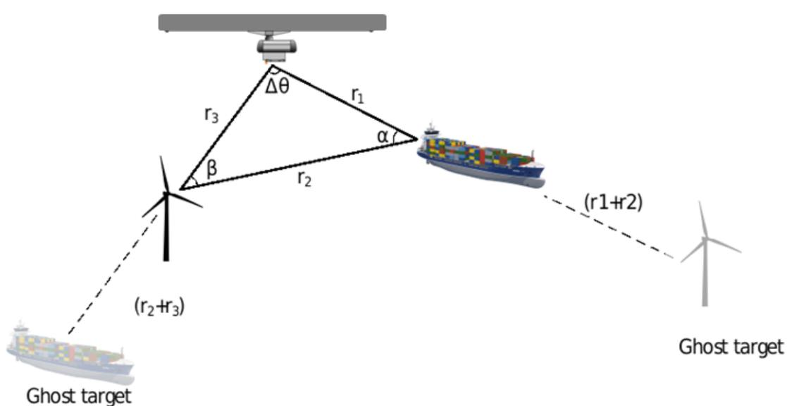
Figure 18 Multipath propagation resulting in Ghost images
