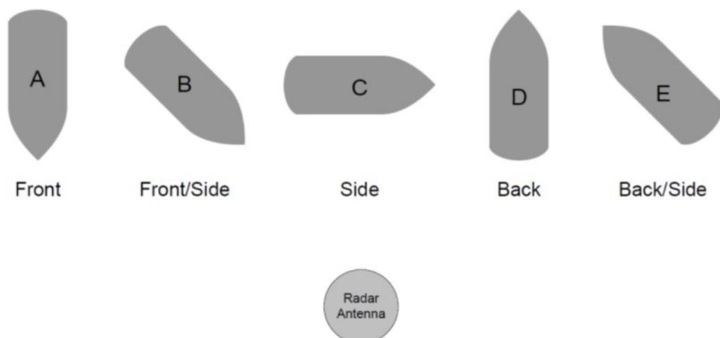
Figure 25 Target aspect angle relative to the radar antenna
