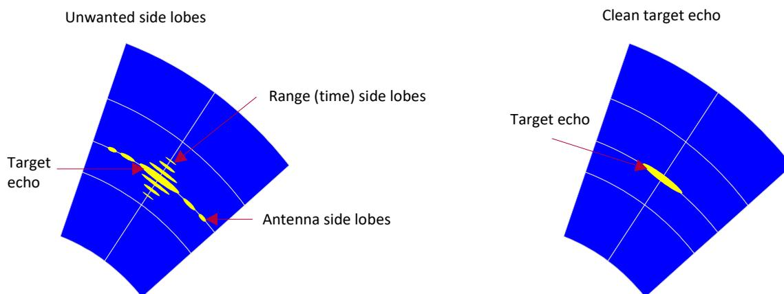
Figure 12 Range and antenna (azimuth) side lobe effects
