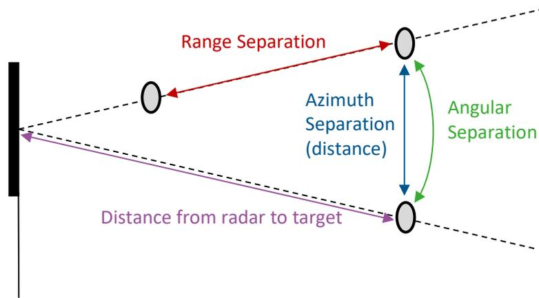
Figure 3 Target separation
