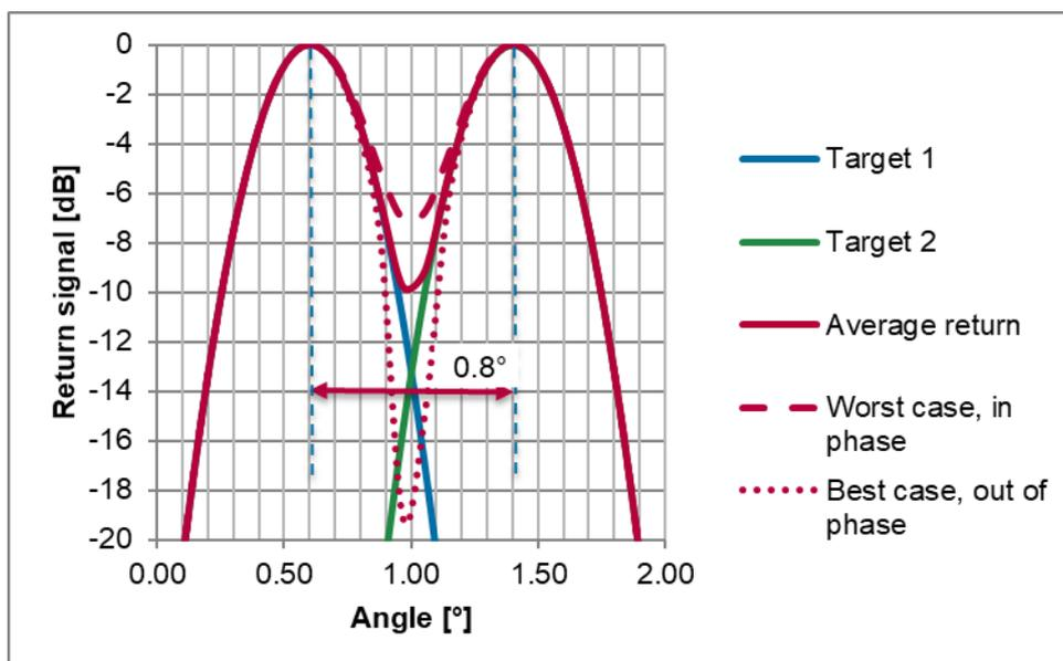
Figure 8 Example of Return from two identical targets placed at the  $0.6^\circ$  and  $1.4^\circ$  angles
