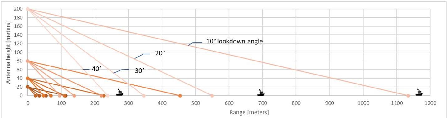
Figure 4 Minimum detection range as a function of antenna height and lookdown angle.
