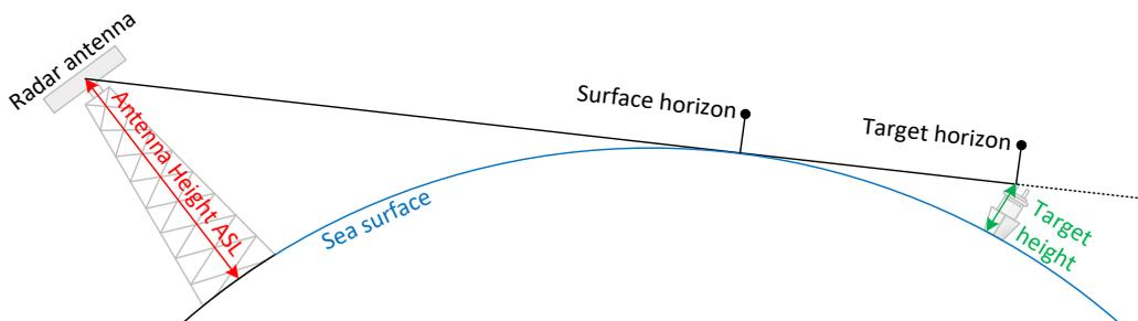
Figure 5 Geometry, antenna height and target height
