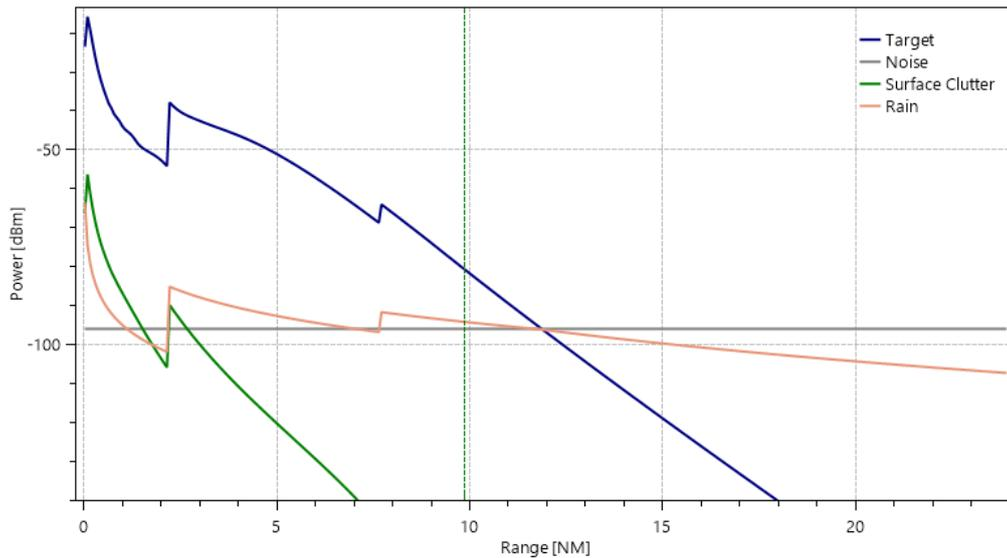
Figure 6 Example of received power versus range
