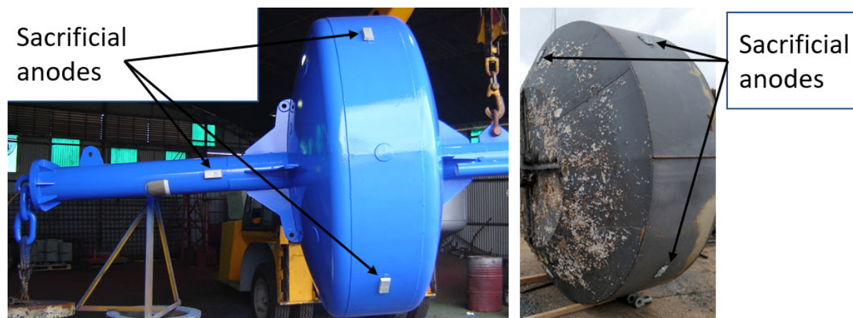
Figure 24 Sacrificial anodes before and after of spar buoy installation
