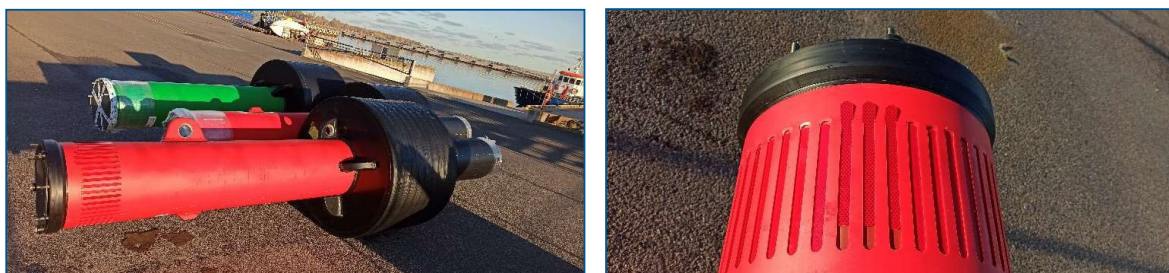
Figure 16 Example of recessed retroreflective film
